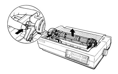
2. Replace the paper eject guide by fitting its notches onto the pins inside of the printer at each side, then tilting the guide back slightly.
